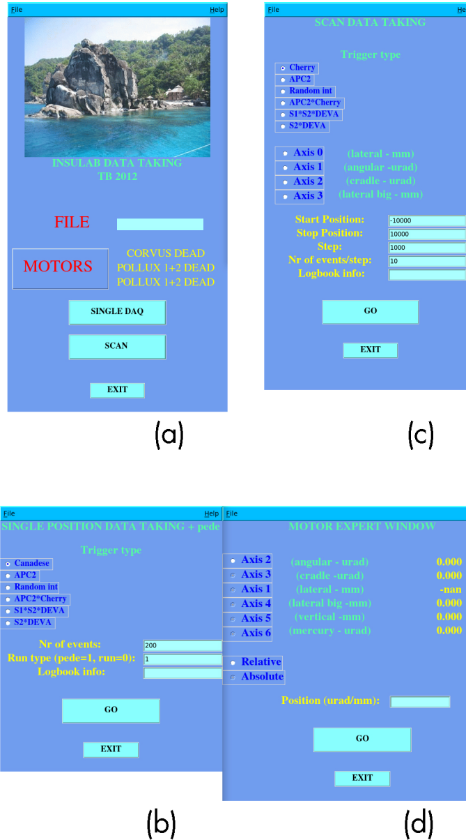
Figure 3.10: Screenshots of the DAQ software windows: (a) main window, (b) single DAQ tab, (c) scan of a goniometer stage and (d) window for the manual movement of the goniometer stages.
