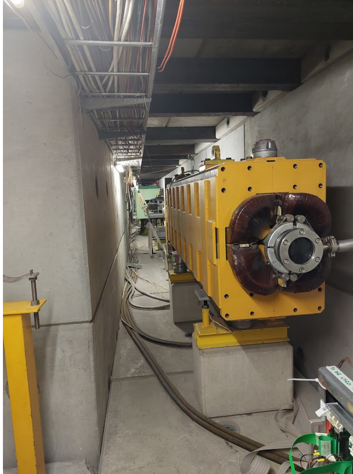
Figure 1.8: Photo of the QNL 427 quadrupole focussing magnet installed in the H8 beamline inside PPE128 at CERN.
